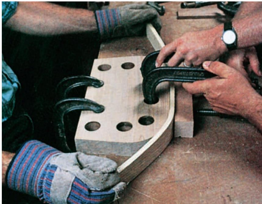
**Figure 1:** Once the steamer was working properly and the author's air-dried stock was good and hot, the ash bent quite easily—a bending strap wasn't even necessary.
