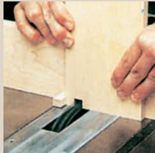
**Step 3:** Position the box side as shown above to make the first cut. Then place the cut you just made over the guide pin to automatically index the next cut.
