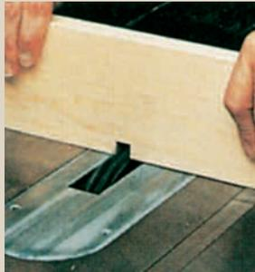
**Step 1:** Install a 1/2" dado blade and a tall miter fence. When you're sure the fence is square to the blade, make one pass with the blade raised to 9/16".
