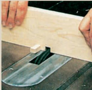
**Step 2:** Glue a 1/2" x 9/16" x 2" guide pin in the dado you just made and reposition the fence 1" to the right. Make a second pass, leaving a 1/2" gap between cuts.
